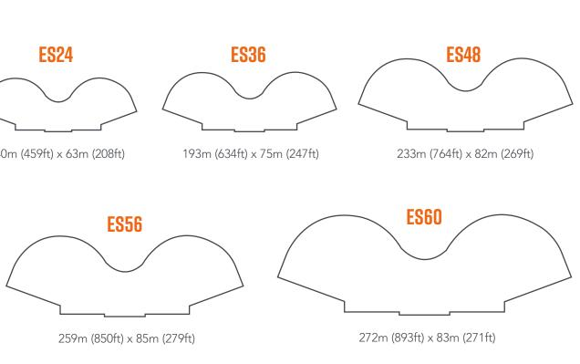
ES24 through ES60 are primary sizings, although we can accommodate lagoons larger and smaller or with any number of caissons in between.
